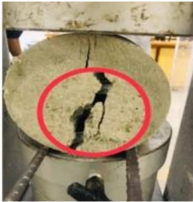
Figure 4 Bridging effect of fiber.
