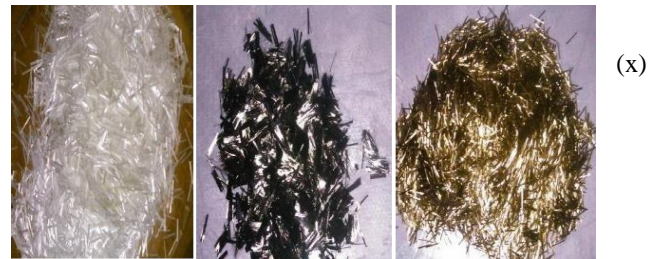
Fig.1 (X) Glass Fiber (Y) Carbon Fiber (Z) Basalt Fiber
