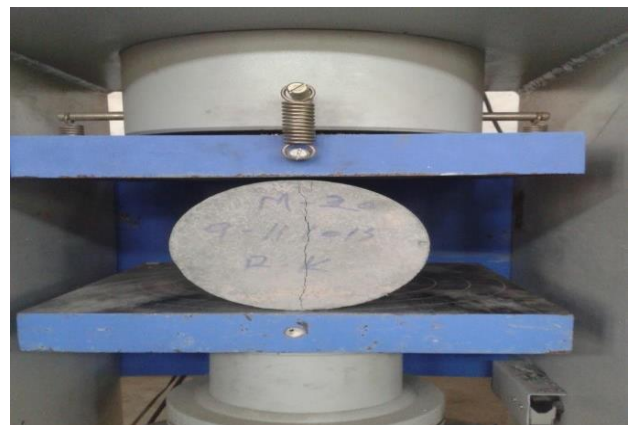
Fig. 5: Test set up for Split Tensile Test
