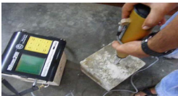
Fig. 7 Static UPV Test on Stone
