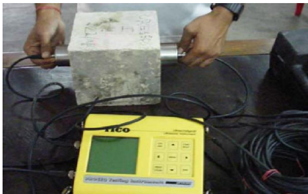
Fig. 6 Static UPV Test on Cubes
