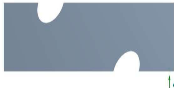
Figure 3: CAD model of plate fin with elliptical tube inclined at 30° heat exchanger
