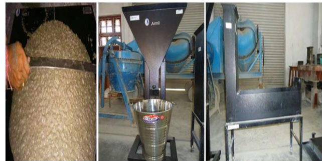
Figure-3: (A) Slump flow test, (B) V-Funnel test, (C) L-Box test
