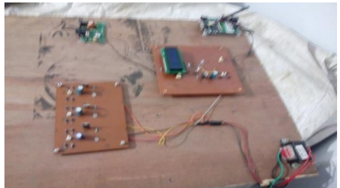
Display and operation of Transformer fault detection on PCB.
