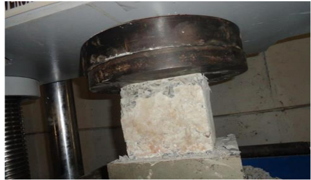
Figure 2: Compressive Strength Test
